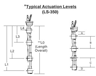
\* Actuation level distances and L<sub>o</sub> (overall unit length) are measured from inner surfaces of mounting.
